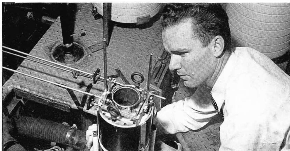
Inspecting the final stage is Mr. Irvin Martin, a member of the power-tube group. The input cavity and a portion of the output stage are clearly visible.
