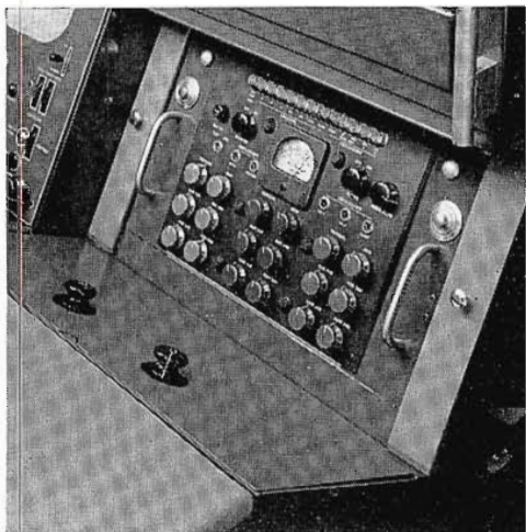
FIG. 2. The processing amplifier in its console housing. This is used in majority of installations.
