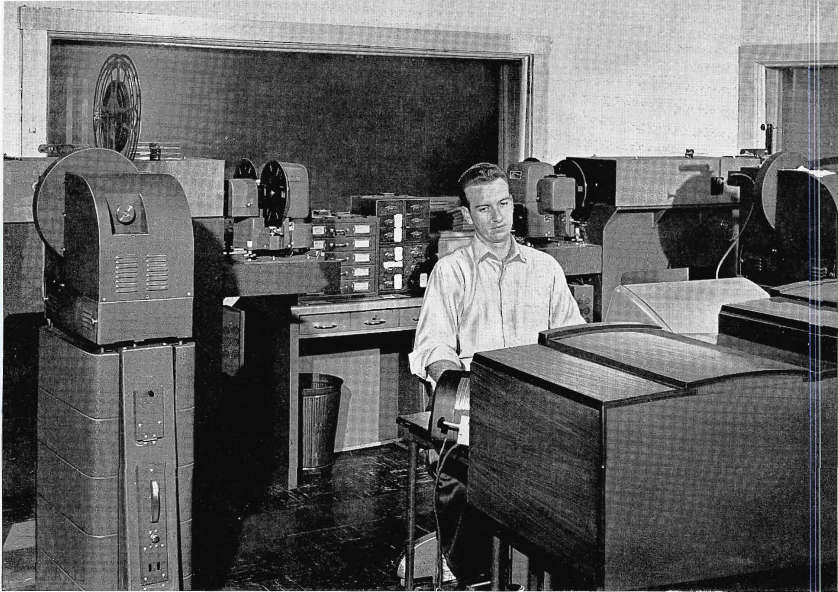
RCA Vidicon Film Cameras installed in the WAAM-TV projection room. Savings afforded in conversion permit the use of two independent film chains for ease of operation as well as provision for preview and auditioning. When the equipment was purchased, the projection room was rebuilt to provide space for both monochrome and future color film equipment.
