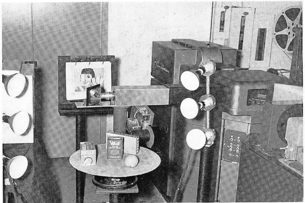
FIG. 6. Test setup showing arrangement of 500 watt photoflood lamps on display table and 7½ by 10 inch color opaques behind mirror.
